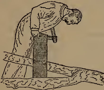
Fig. 51.—Springing the Rift
